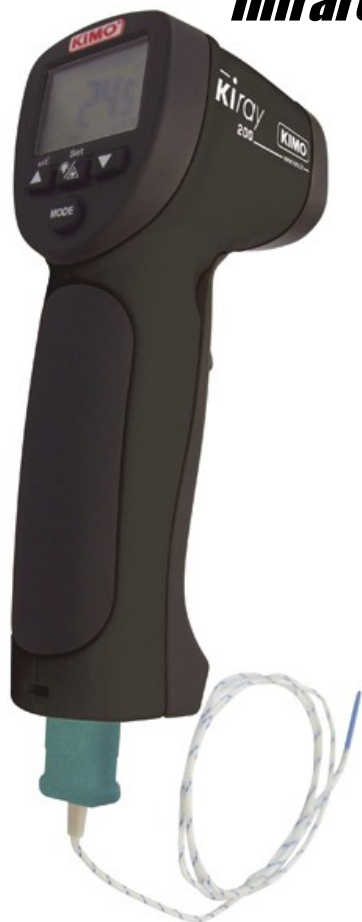
Supplied with thermocouple K probe
